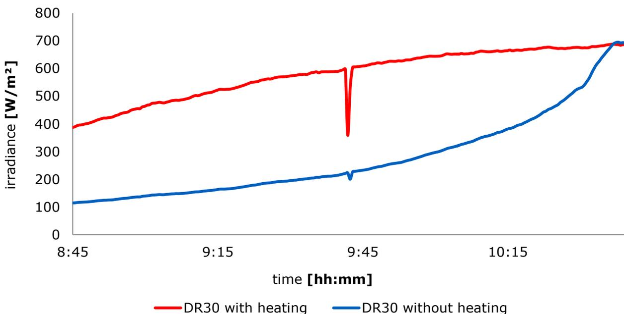
**Figure 7** comparison of the measured data with and without heating on a typical winter morning. The unheated DR30 has dew on its front window and strongly underestimates the incoming irradiance. At around 10:30 the dew evaporates. Real measured data from Delft, the Netherlands.
