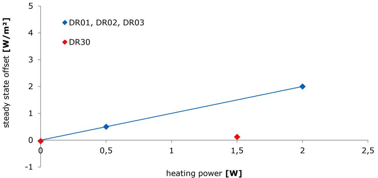
**Figure 6** the offset of DR30 when heating is much improved relative to the older DR01, DR02 and DR03 models. DR30 has a 1.5 W heater and produces a negligible offset. The older models had offsets of the order of 2 W/m<sup>2</sup> at the same heating levels. In addition, the temperature of the front window of DR30 is 4 times higher than that of the older models, at the same heating power.
