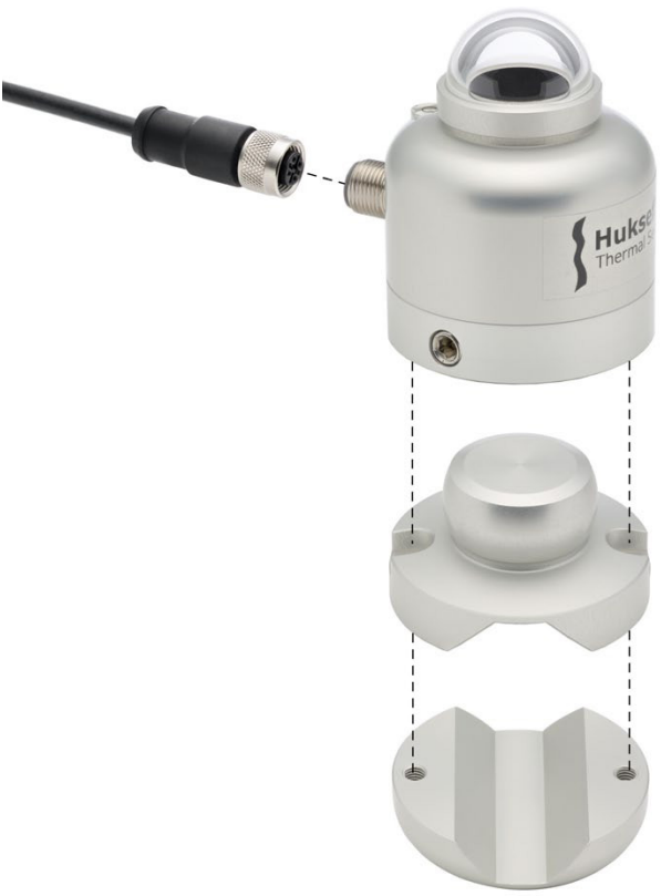
Figure 3 'Exploded view' of SV-SR05 The optional ball levelling and tube mount allow for easy installation. The cable (standard 3 m) has an M12-A connector.
