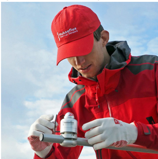
Figure 2 Easy levelling of SV-SR05 on its tube mount with ball levelling
